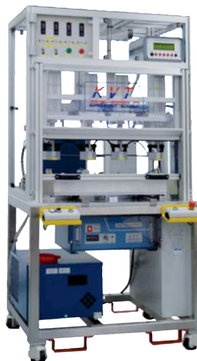
ERW thermal installation machine to embed four inserts into a boot handle
